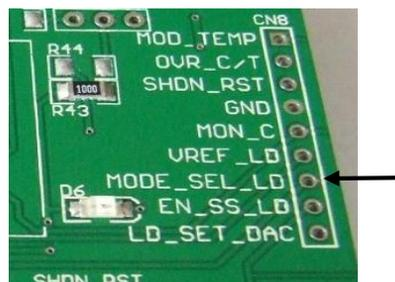
Alternatively, Mode control can be set by an external system. With the link in the CC/External position the control line can be accessed via Mod\_SEL\_LD at CN8. This node should be pulled high for Constant Power mode, and released, or pulled down, for Constant Current mode. (an internal pull-down inside the module sets Constant Current as the default mode).
